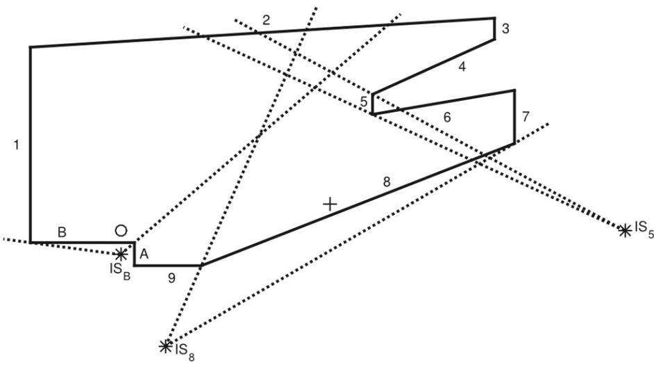
Figure 5: An example of the image-source style of beam tracing, from [Savioja and Svensson, 2015].
