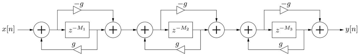
Figure 9: Cascaded Schroeder allpass sections.
