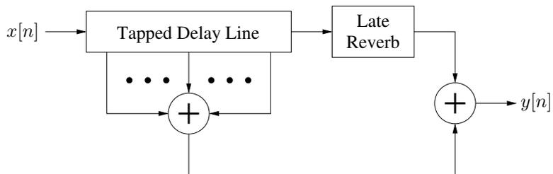
Figure 8: Early reverberation implemented with a tapped delay line, followed by a late reverberation processing block.
