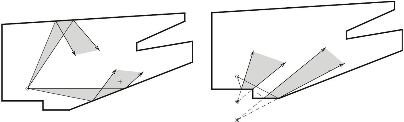
Figure 4: An example of the ray-tracing style of beam tracing, from [Savioja and Svensson, 2015].
