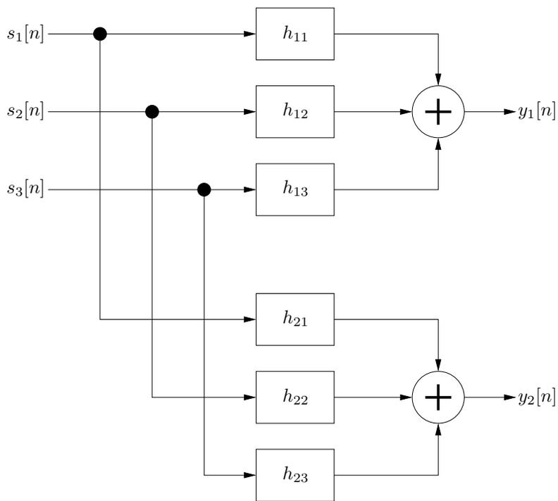
Figure 7: Transfer function approach to reverberation simulation for three sources and one listener.
