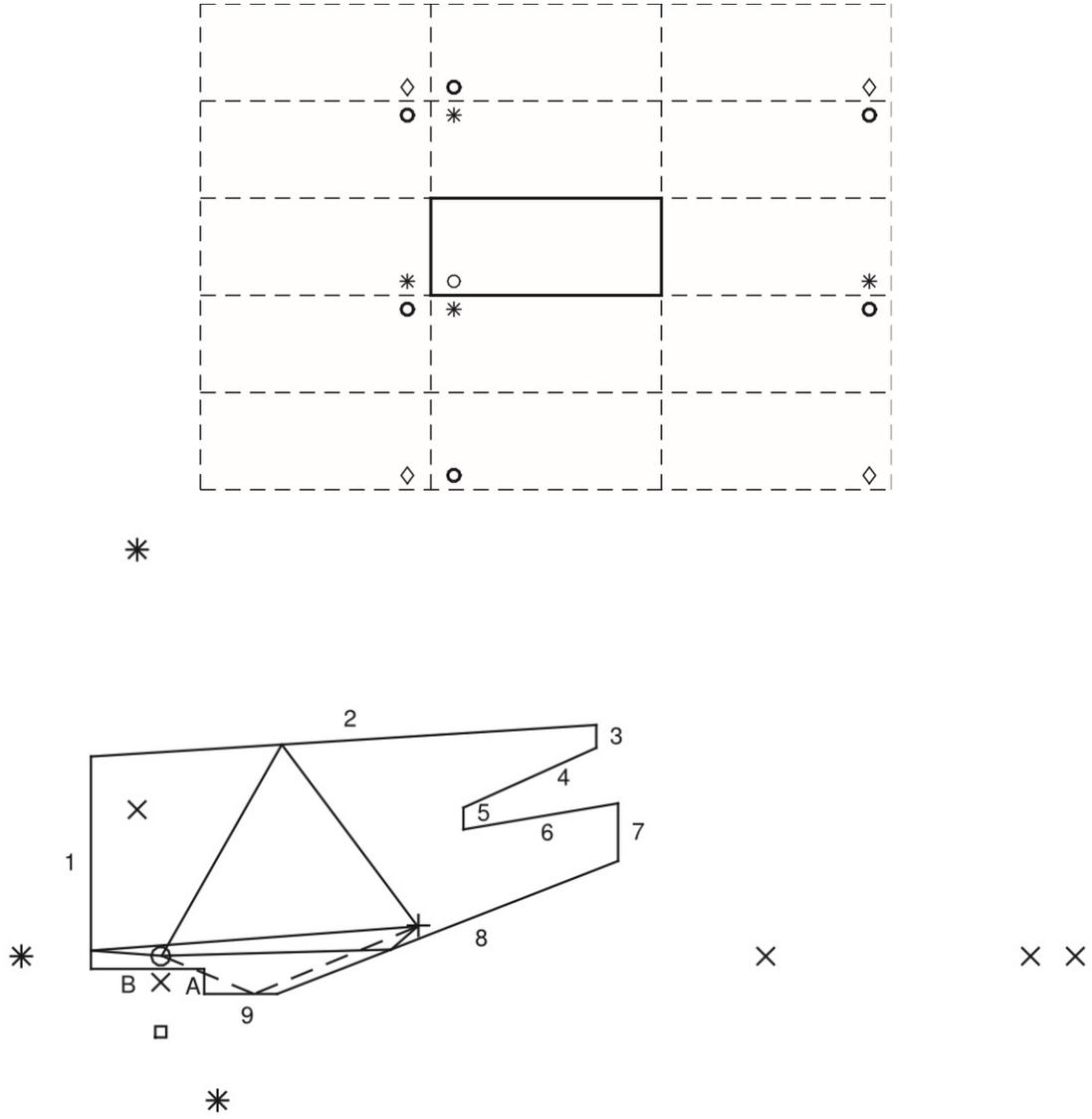
Figure 2: Image-source representation of a shoebox-shaped room (left) and a more complex geometry (right), from [Savioja and Svensson, 2015]. Original sources are designated by ◦, first-order ISs with \*, second-order ISs with ◦, and third-order ISs with ◊. For the right figure, the receiver is designated with +, ISs with reflection points outside the polygon by × and an IS with a valid reflection point but obstructed path with ◻.
