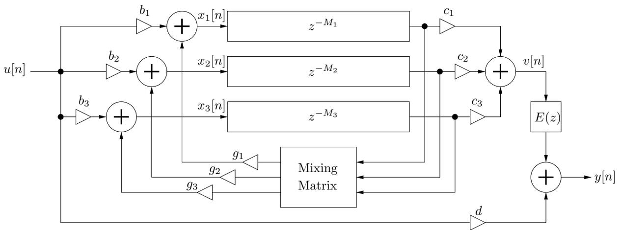
Figure 12: A feedback delay network structure proposed for artificial reverberation by Jot [1992].
