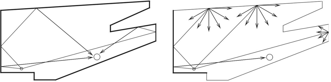
Figure 3: Specular (left) and diffuse reflection (right) ray tracing examples, from [Savioja and Svensson, 2015].
