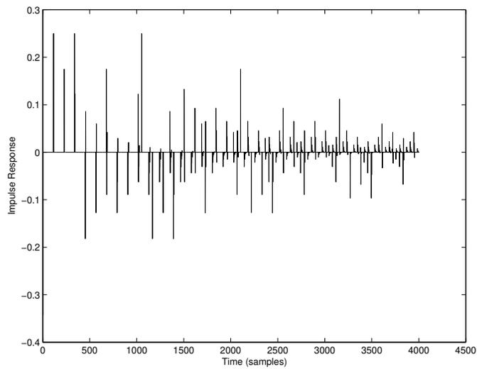
Figure 10: Impulse response of three cascaded Schroeder allpass sections ( $g = 0.7$  and  $M_i = [113, 337, 1051]$ ).
