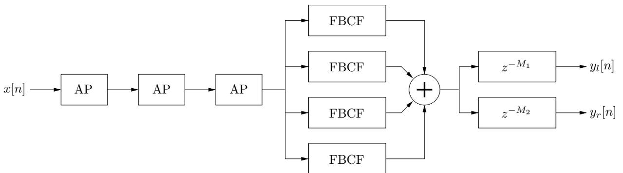
Figure 11: The JCRRev reverberator from CCRMA (based on Schroeder/Moorer).
