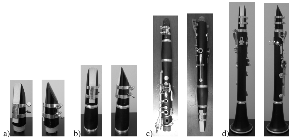
Figure 1: Two views of each of four (4) clarinet configurations: a) mouthpiece alone, b) mouthpiece with barrel, c) mouthpiece with upper joint (upper demi-clarinet) and d) mouthpiece with lower joint and bell (lower demi-clarinet).
