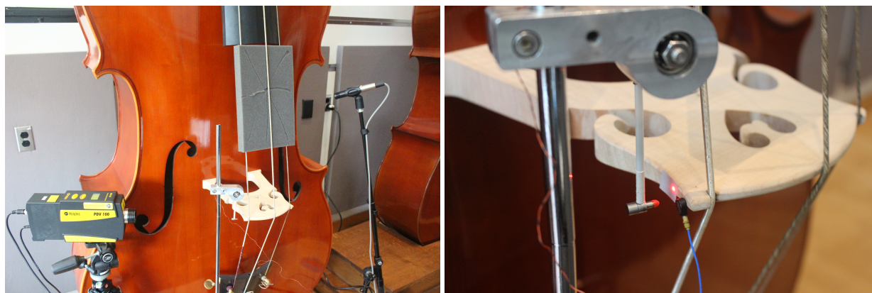
Figure 4: Admittance measurement setup for an octobass.
