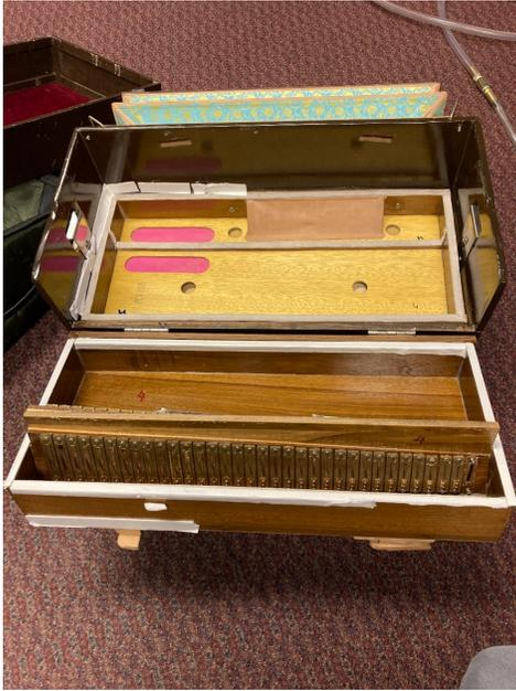
(a) Reed chamber of a harmonium. The four small holes connect the reed chamber with the spring-piston chamber
