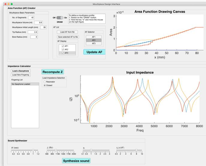
Fig. C.2: Comparison of AFs and closed mouthpiece input impedances.
