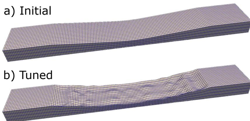
Figure 4.6: Example rosewood bar tuned to the typical 1:4:10 ratios using a **moderate cutaway** as its initial input geometry. (a) Initial geometry. (b) Tuned geometry.
