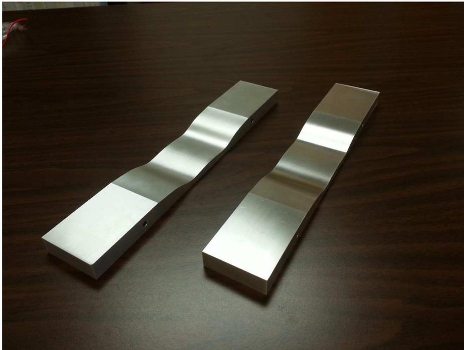
Figure 2.5: Vibraphone bars tuned to musical note A4 and fabricated via CNC mill per [Kirkland and Moradi \(2016\)](#).
