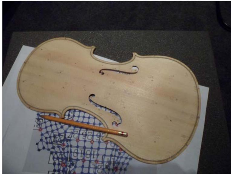
**Fig. 3.12** Marked points on the spruce plate
