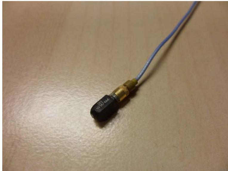
**Fig. 3.10** Accelerometer Model 352C23/NC
