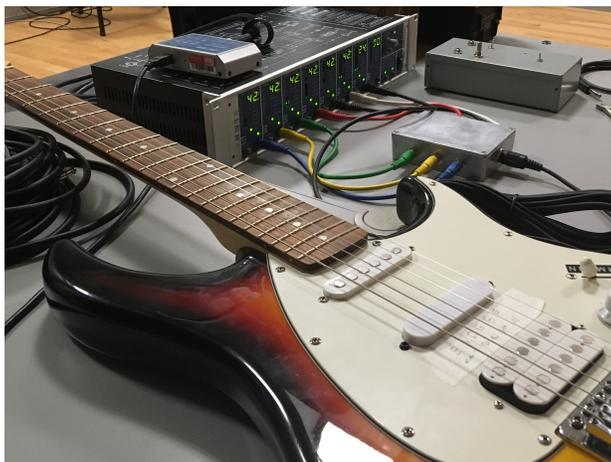
Figure 3.1: *Hexaphonic recording setup. The hexaphonic pickup is the middle pickup. The color patch cables connect the breakout box to channels 1 through 6. An additional patch cable connects the mono pickup to input channel 7.*
