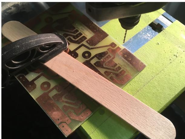
Figure 5.2: *The etched board being drilled prior to being cut into four Distorter R VIII circuits.*
