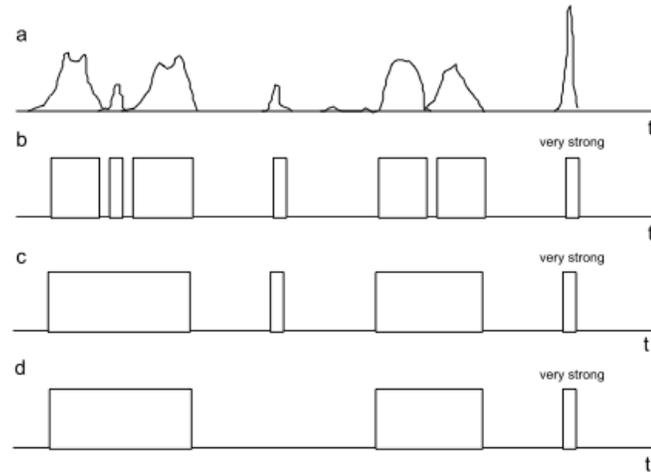
**Fig. 4.24** Pause detection steps from Li et al. (2001): (1) short time energy of input signal; (b) initial result for candidate signal segments; (c) result after fill-in step; (d) result after throwaway step.
