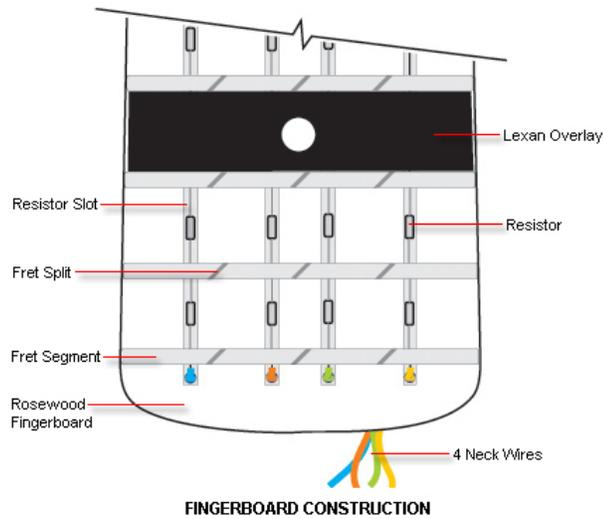
**Fig. 4.11** Diagram of the wired frets used in the Industrial Radio MIDI Bass from (Industrial Radio 2010)
