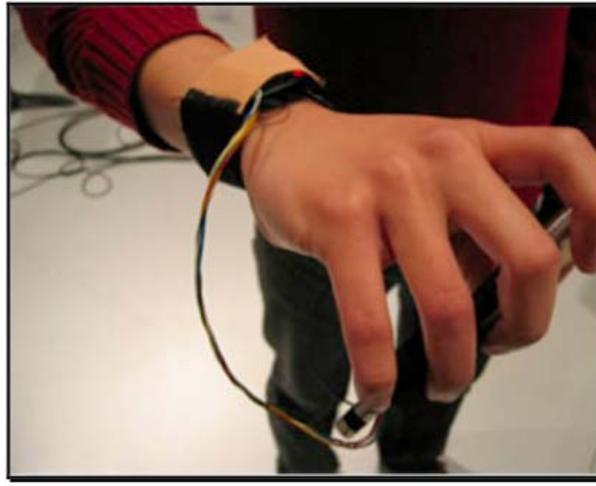
**Fig. 2.21** Wireless gesture sensor attached to student's wrist and violin from (Ng 2008b)
