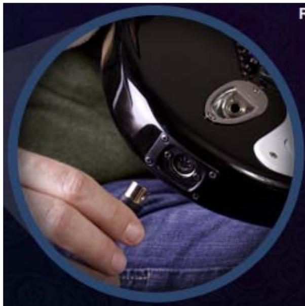
**Fig. 4.15** MIDI Output jack for the Squier by Fender Stratocaster Guitar Controller from (Fender 2011)
