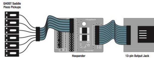
**Fig. 4.6** Overview of the Graph Tech Ghost Pickup System from (Graph Tech Guitar Labs 2010)
