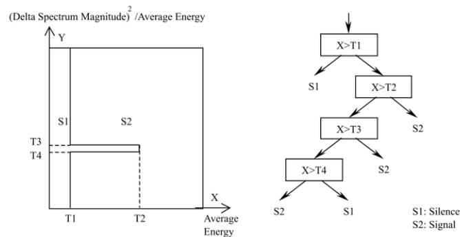
**Fig. 4.23** Two-dimensional partitioned space and its corresponding decision tree. Where T1, T2, T3, and T4 are threshold values. From (Li et al. 2001)
