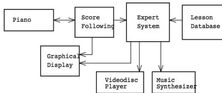
**Fig. 2.1** Piano Tutor's principle components from (Dannenberget al. 1990)
