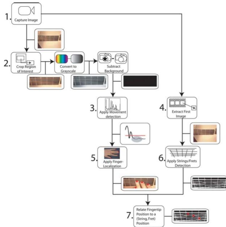
Fig. 4.18 Prototype algorithm for fingering recognition by Burns (2006)
