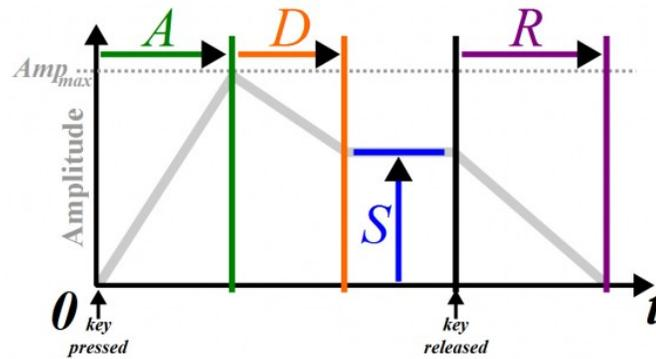
**Fig. 4.21** Basic contour of the sound produced by a musical instrument as delineated by its attack (A), decay (D), sustain (S) and release (R). From (*ADSR Envelope*)
