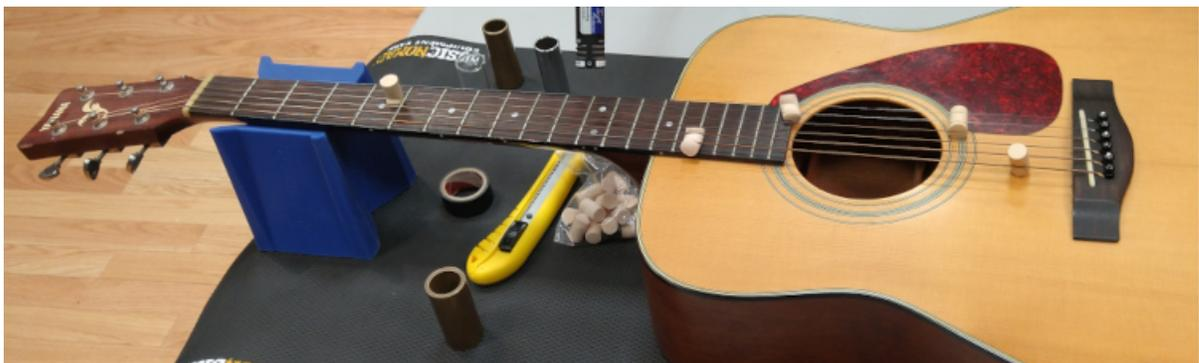
**Fig. 5.3** The setup used to confirm longitudinal-to-transverse coupling. Ear plugs are used to mute strings not being measured.
