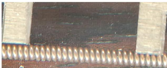
**Fig. 5.2** The E-string winding density measurement. The distance between the inner edges of the caliper is 1 cm. Approximately 20 windings lie on this distance.
