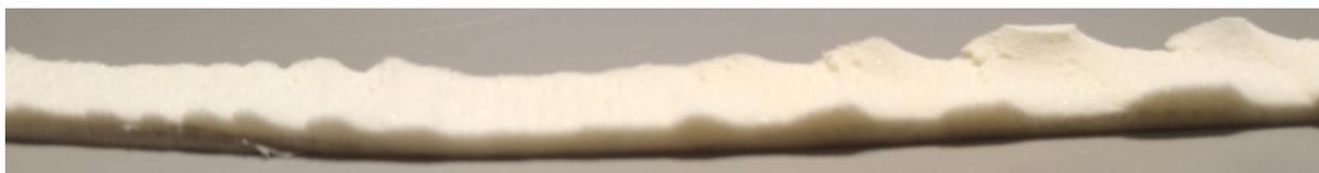
**Fig. 5.7** A failed attempt to reduce the thickness of the foam.
