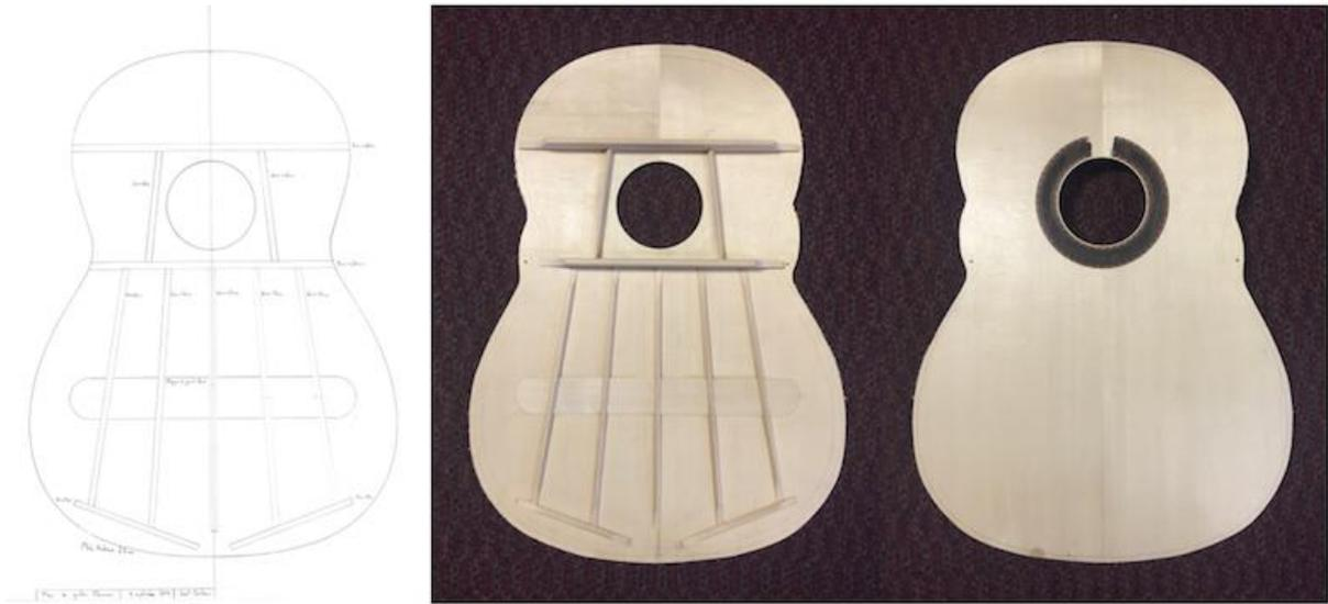
Figure 3.6: Left: the drawing of the soundboard. Centre: the braces behind the wooden soundboard. Right: The front side of the wooden soundboard. The top plate is made from Picea Abie, and the braces from Sitka Spruce.
