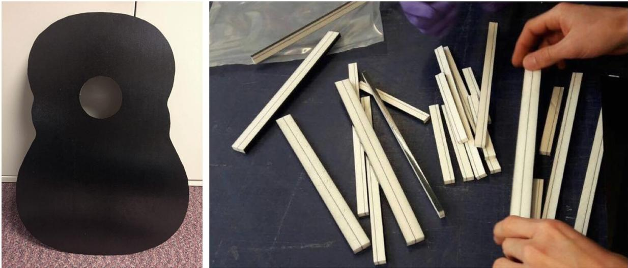
Figure 3.24: The manufactured composite top plate and the braces.
