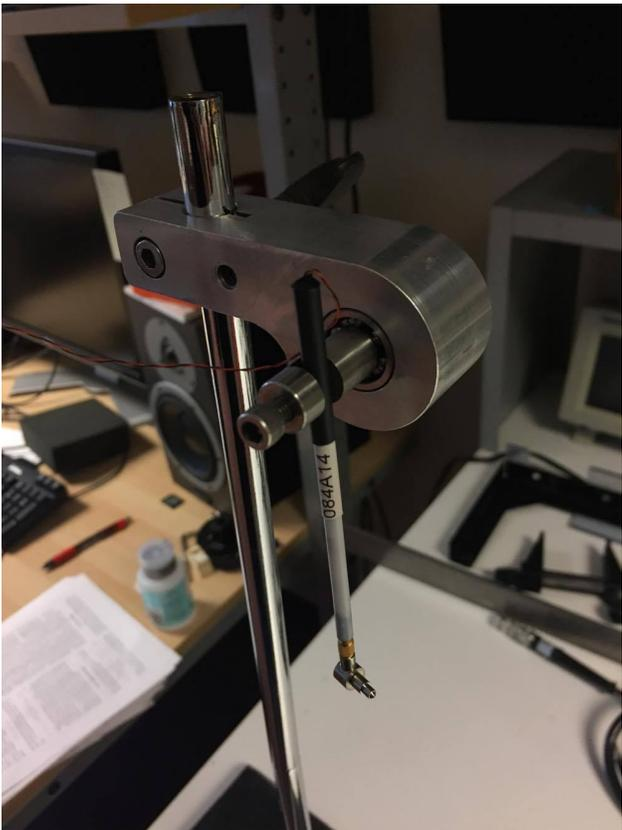
Figure 3.2: The PCB 084A14 miniature hammer.
