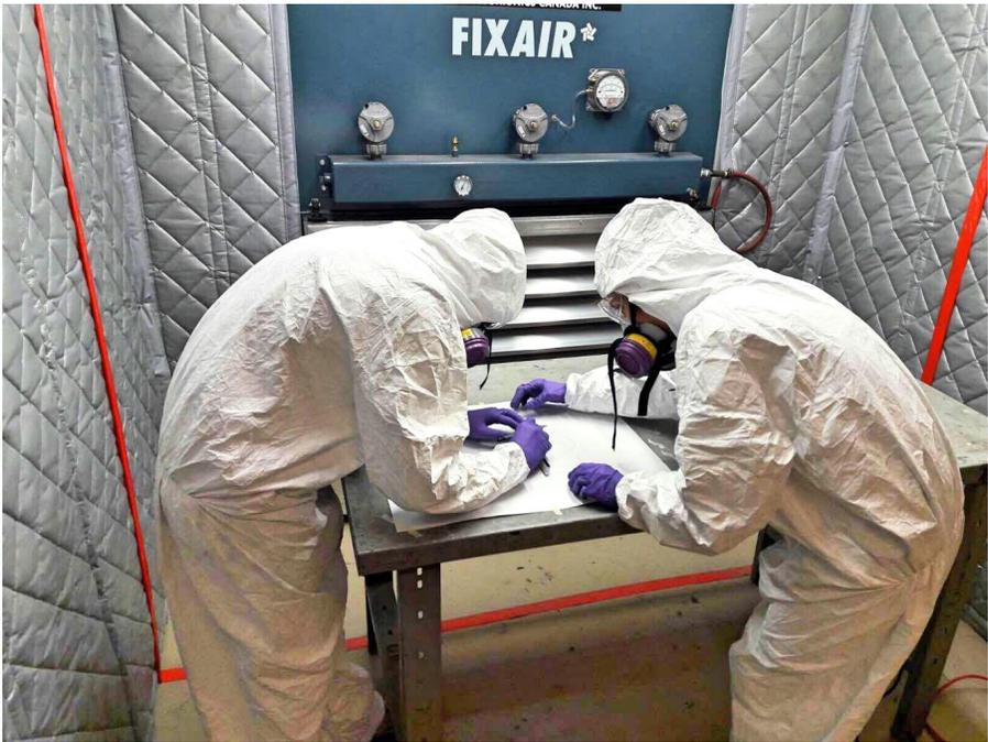
Figure 3.22: The booth designated for dry cutting carbon fibres and composites.
