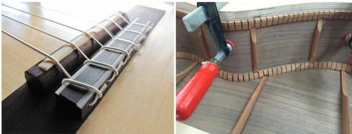
Figure 2.9: Left: The strings tied to the bridge [33]. Notice the compensated saddle between the strings and the bridge. Right: The wooden slots around the ribs are the lining.
