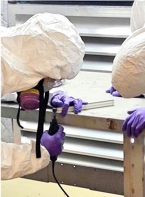
Figure 3.23: Dry cutting the edge of the braces using the Dremel.
