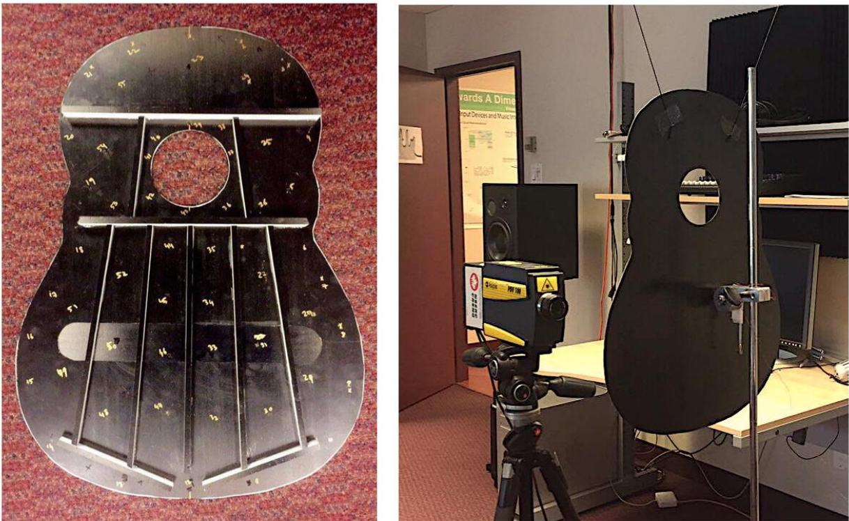
Figure 3.27: Left: Measurement points marked on the composite soundboard. Right: The measurement setup for the composite soundboard.
