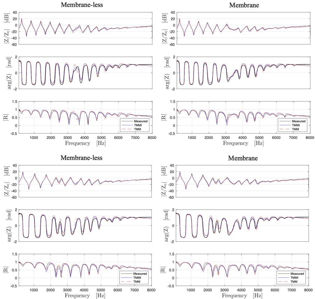
**Figure 5: Normalized input impedance modulus and phase and reflection coefficient modulus for the XXXXXX (top) and XXXXOO (bottom) fingering of the dizi. The black curves represent measurement data, the blue curves represent TMMI data and the red curves represent TMM data. The top two graphs correspond to the membrane-less dizi, and the bottom two graphs correspond to the membrane dizi.**
