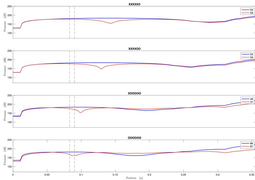
**Figure 8: Relative standing pressure wave distribution in the air column of the dizi with the membrane. From top to bottom, the blue curves correspond to the notes D5, E5, A6, and B6 (the first octave), and the red curves for D6, E6, A7, and B7 (the second octave). The abscissa represents the distance from the cork, and the ordinate represents the sound pressure level. The section between the gray dotted lines is the position of the membrane hole.**
