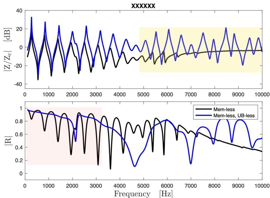
**Figure 6:** Normalized impedance modulus and reflection coefficient modulus for the XXXXXX fingering of the dizi, calculated using the TMMI. The black curves represent no membrane and the blue curves represent no membrane and no upstream branch.
