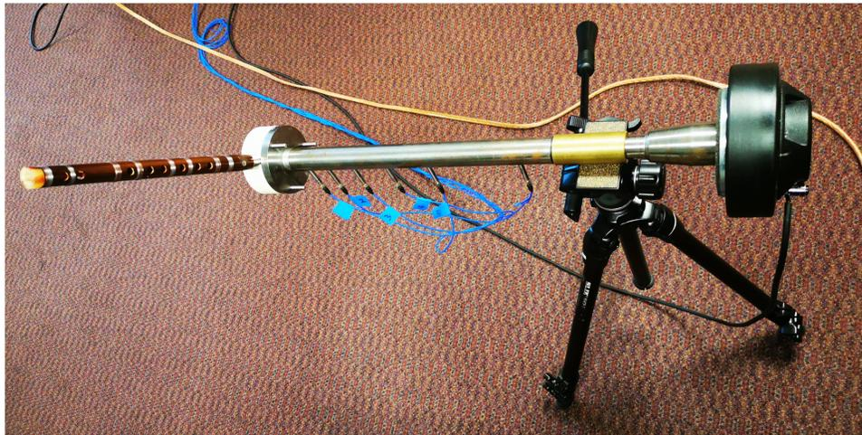
*Figure 3: Image of the impedance tube.*
