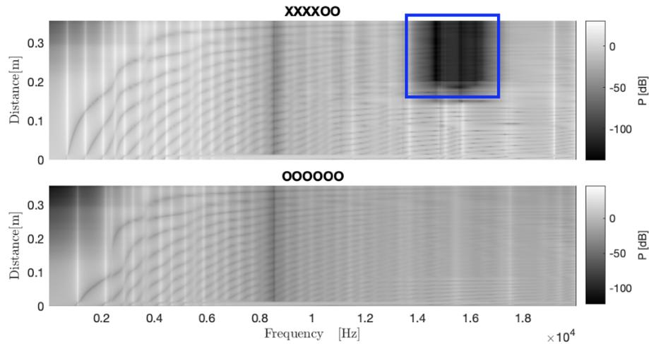
**Figure 11:** Normalized pressure map of dizi without membrane. The horizontal axis shows the frequency, and the vertical axis represents the position along the bore relative to the cork. The top is the result of XXXXOO fingering and the bottom is for OOOOOO fingering.
