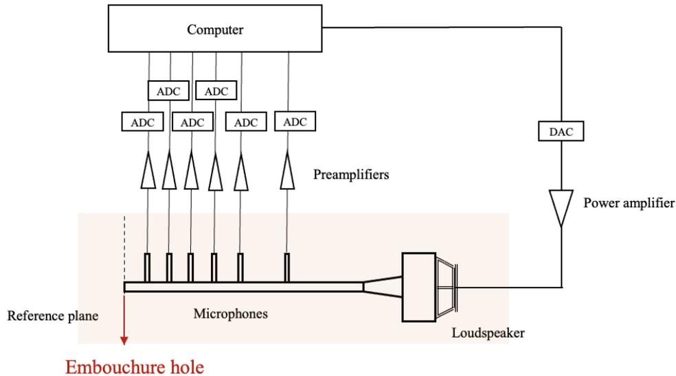
*Figure 2: Schematic of the measurement system.*
