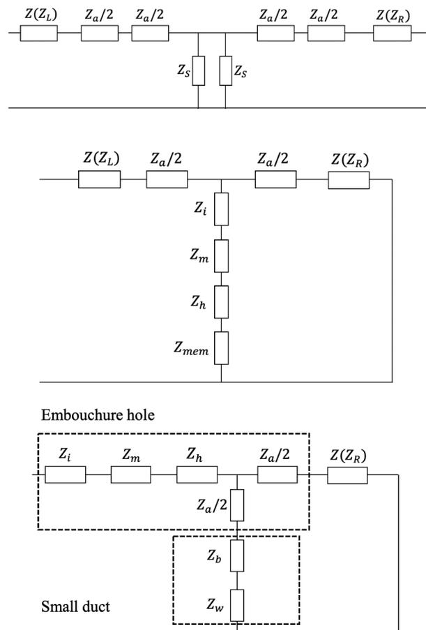
**Figure 4: Equivalent circuits representations for the back end-holes (top), membrane hole (middle), and embouchure hole (bottom).**
