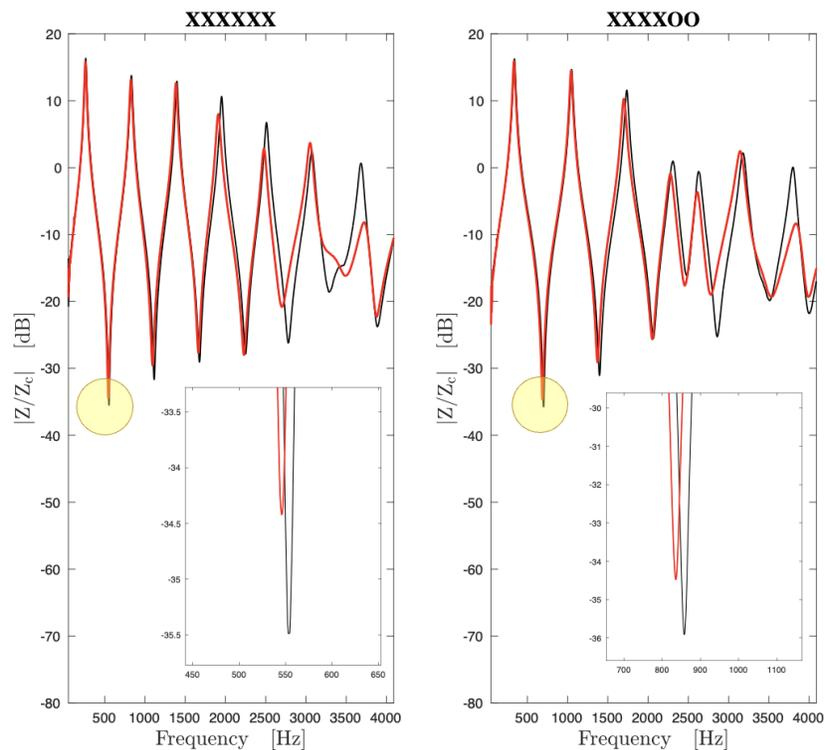
**Figure 7: Measured normalized impedance modulus of the dizi, corresponding to XXXXXX fingering on the left and XXOOO fingering on the right. The black curves represent membrane-less dizi, the red curves represent membrane dizi and the first minima are zoomed in.**
