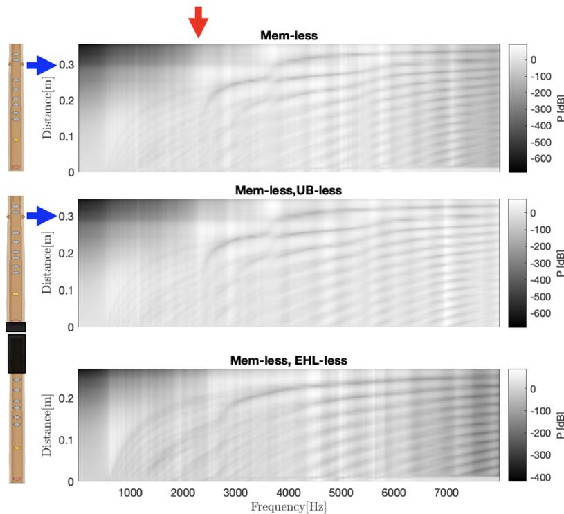
**Figure 12:** Normalized added pressure map of dizi without membrane for fingerings from XXXXXX to OOOOOO. The upper map is for the whole dizi, the middle is for the dizi without the upstream branch, and the lower is for the dizi without the EHL.
