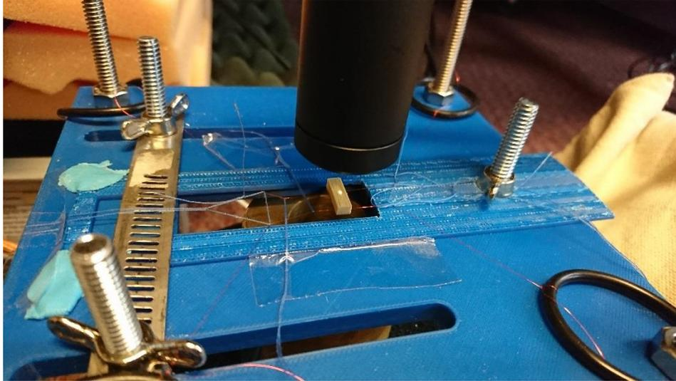
**Figure 3: Experimental setup for internal friction measurements depicting the sample, confocal displacement sensor and compression driver.**
