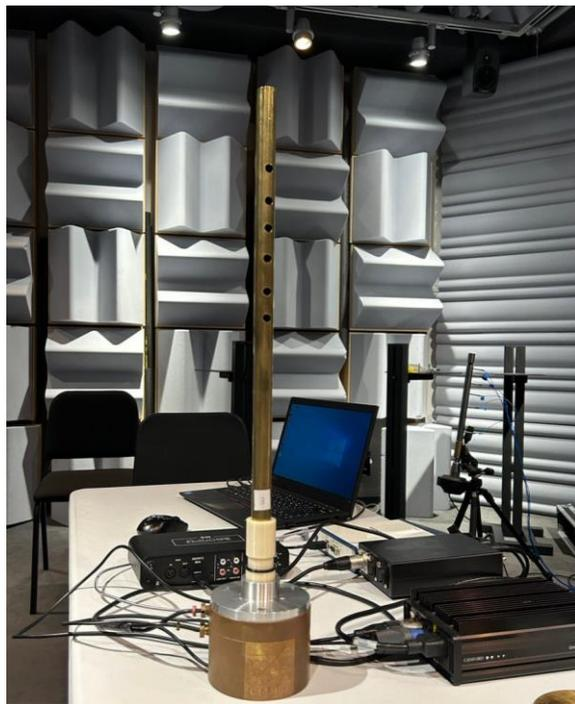
**Figure 4** Impedance measurement of şimşal with *CapturZ*.
