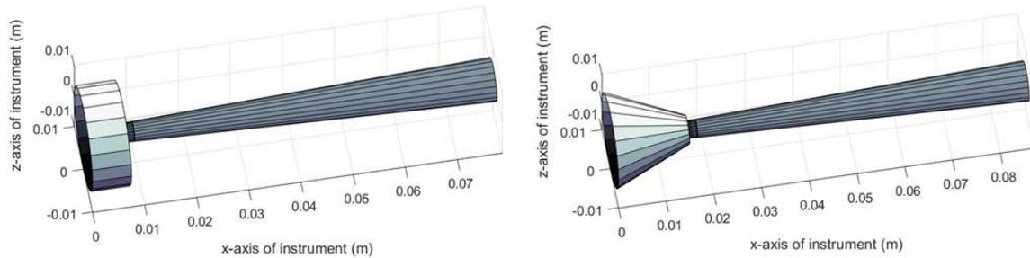
**Figure 4:** Wire diagrams of a cylindrical (left) and conical (right) approximation of the cup of the 5C mouthpiece described in §3.B.ii.
