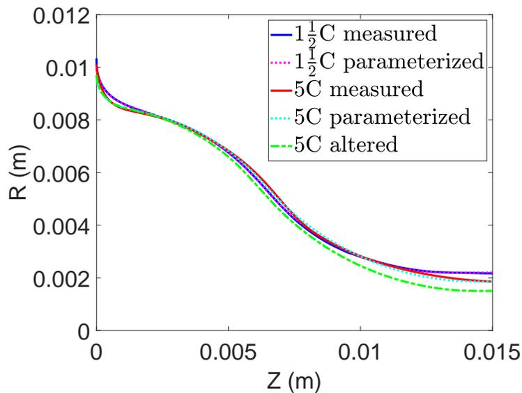
Figure 3: Measured geometries and parameterizations of Vincent Bach 5C and  $1\frac{1}{2}C$  trumpet mouthpieces, and a modification of the 5C mouthpiece parameterization produced by narrowing just the throat radius and leaving all other parameters unchanged.  $R$  is the radial dimension and  $Z$  is the dimension along the axis.
