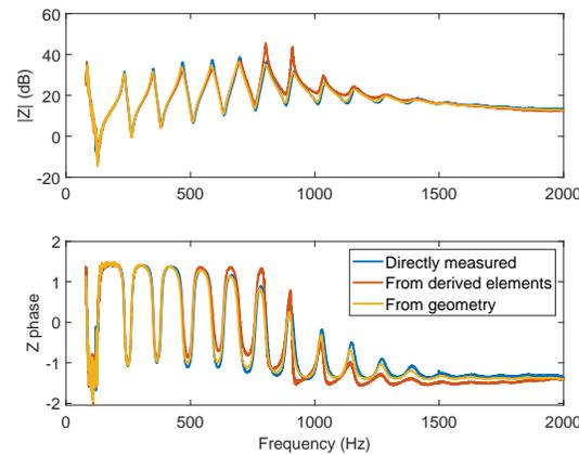
**Figure 9:** A comparison of the trumpet impedance (magnitude and phase) calculated from derived TMM elements (from impedance measurements involving the mouthpiece, as described in the text) and a measured trumpet load impedance, from a TMM calculation combined with the same load impedance, and from a direct impedance measurement of the same mouthpiece and trumpet.
