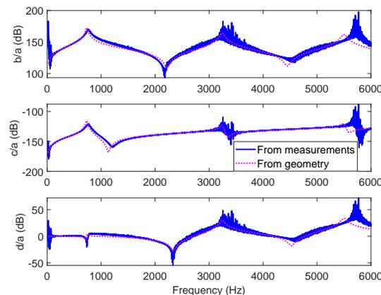
**Figure 8:** A comparison of the TMM element ratios of a mouthpiece from impedance measurements and calculated from the geometry.
