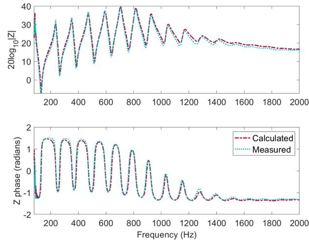
**Figure 6:** A comparison of the impedance (magnitude and phase) determined from a TMM calculation from the mouthpiece geometry combined with the trumpet load impedance (described in §3.A), and a direct impedance measurement of the same trumpet and mouthpiece combination.
