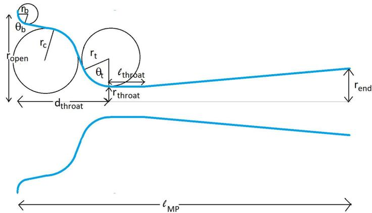
Figure 2: Proposed parameterization of a trumpet mouthpiece.
