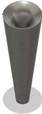
*Figure 5: Wire diagram of the 3D printed trumpet bell shape used for impedance measurements.*
