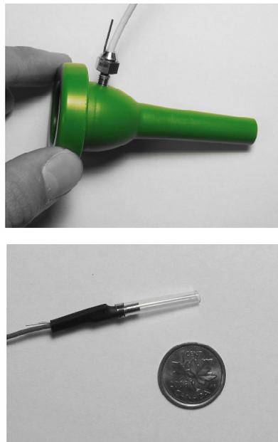
**Figure 1.** Downstream microphone mounted on a plastic mouthpiece (top), upstream microphone inserted into a small silicone tube (bottom).
