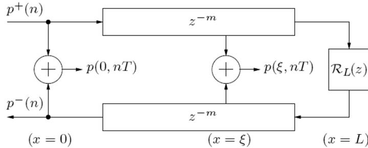
Figure 1: A one-dimensional digital waveguide model of a cylindrical air column.
