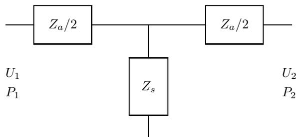
Figure 1:  $T$  section transmission-line element representing the tonehole.
