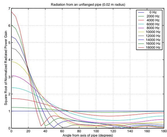
Figure 2: Radiation directivity vs. angle from pipe end.
