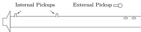
Figure 3: Internal and external pickup locations.
