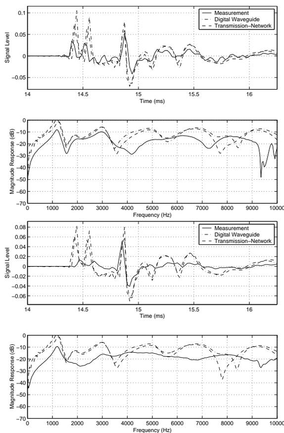
Figure 8: All holes open. Measurement angles: 90° (top) and 270° (bottom).
