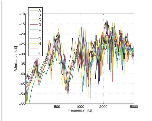
Figure 1. Bridge admittances of the ten violins used in the experiment, obtained by exciting the G-string corner of the bridge with a mini impact-force hammer and measuring the velocity at the E-string corner of the bridge with a laser Doppler vibrometer.
