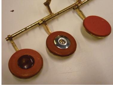
Figure 1: (Color online) Three kinds of pads: with a plastic resonator on the left, with a metal resonator in the middle, and without a resonator on the right.
