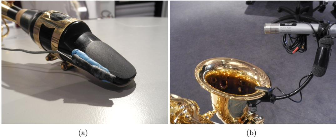
Figure 12: (a) Differential pressure transducer Endevco 8507-C1 used to measure the static pressure in the mouth and (b) Microphone B&K 2669 located at 15 cm from the bell used to measure the radiated pressure.
