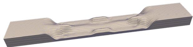
FIG. 6. (Color online) Tuned geometry of model 1(f), a rosewood F3 bar tuned to modal frequency ratios: V1-1, V2-4, V3-10, T1-2, T2-8, L1-6.
