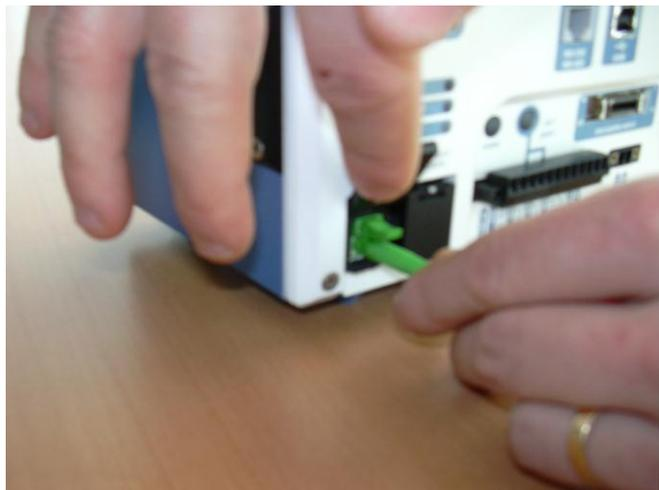
To remove the fiber optics from its socket, first press on the locking lever, then pull the lead out of the socket.
