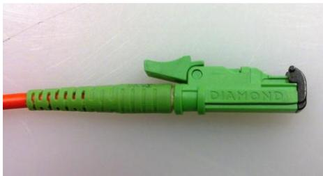
To connect the fiber optics insert the plug into the fiber socket as shown in the figure until a « click » is heard as it locks into position.
