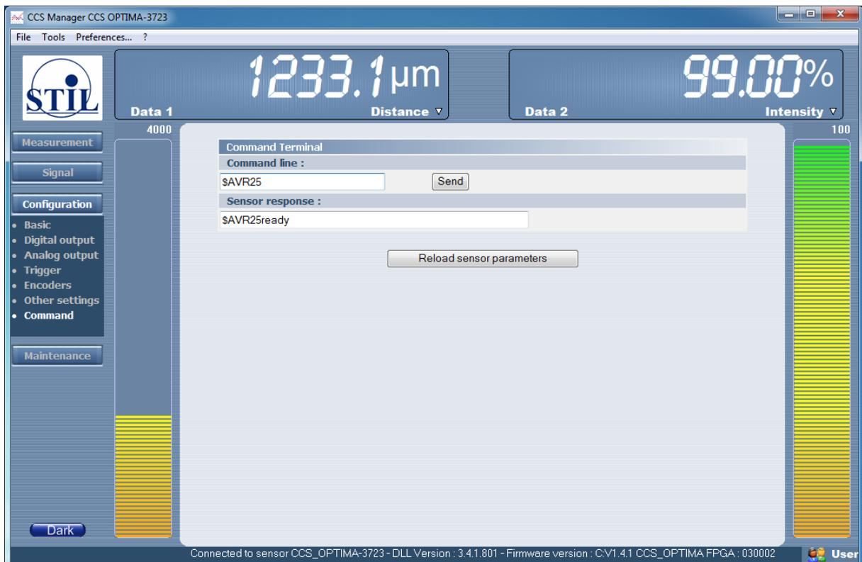
The Terminal allows communicating with the sensor using the specific CCS command language. Commands are described in detail later on in this manual. For the moment, note that commands begin by a \$ sign, comprise 3 upper case letters, and end with the numerical value of the parameter. The sensor echoes the command and then sends “ready”.
