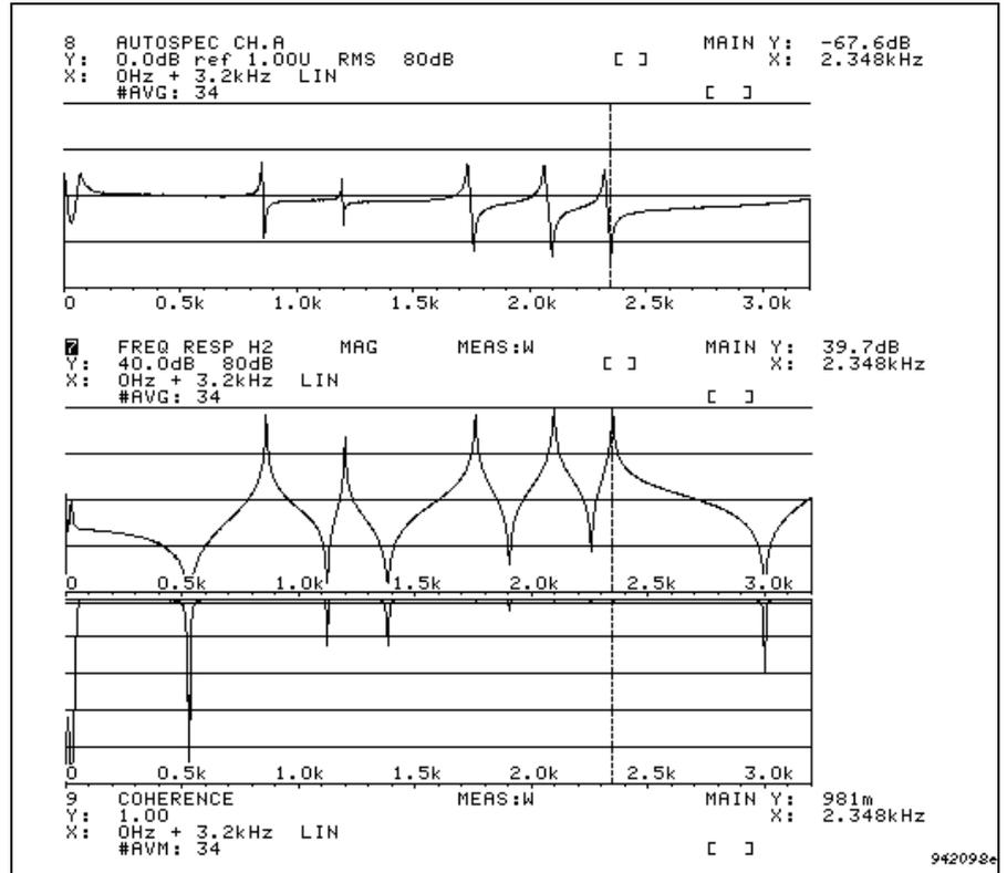
Fig.1 (top) Input force spectrum for pseudo-random excitation. (Bottom) Frequency Response Function and Coherence using pseudo-random excitation. (Measurement performed using the Type 5961 with the Multichannel Analysis System Type 3550)
